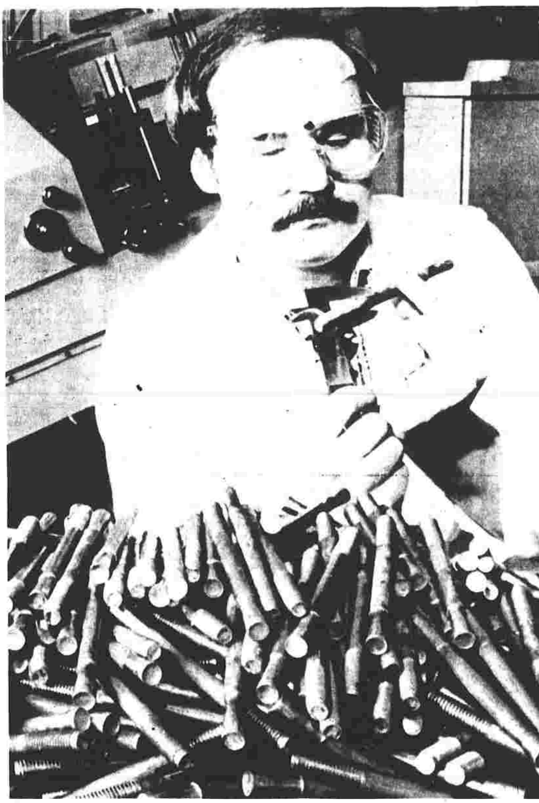
Anchors away Steve Husing uses calipers to measure the diameter of Red Head wedge anchors at ITT Phillips Drill Division in Michigan City, Ind. Wedge anchors are used in heavy duty construction to anchor a large variety of objects to concrete. Applications range from use with electrical; heating, plumbing and ventilating systems to the installation of manufacturing equipment and highway guard rails.
